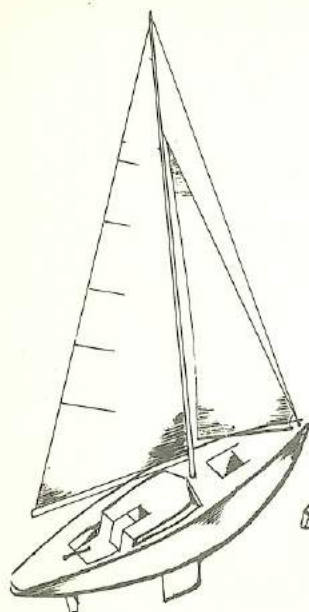
Conventional Boat, Conventional sail, Sloop rigged with three quarter jib
